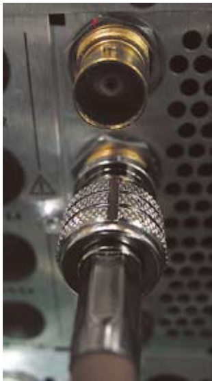
Actual image of the confirmation when BNC Connector has fitted with jack side
